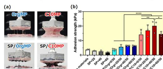
**Fig. 4** (a) Images of tissue adhesion test using porcine stomach submucosal tissue. (b) Maximum adhesion strength of SP/OrgMP and SP/C10MP colloidal gel. \* $p < 0.05$ , \*\* $p < 0.01$ , \*\*\* $p < 0.0001$ .
