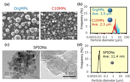
**Fig. 2** (a) SEM images of OrgMPs and C10MPs. (b) Particle size distribution of OrgMPs and C10MPs. (c) TEM image of SPIONs. (d) Particle size distribution of SPIONs.
