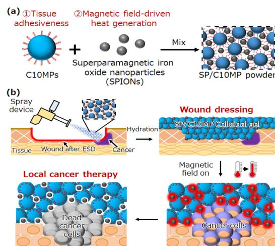
**Fig. 1** (a) Mixing C10MPs and SPIONs to prepare SP/C10MP powder. (b) Application of SP/C10MP colloidal gel for local thermal cancer therapy.
