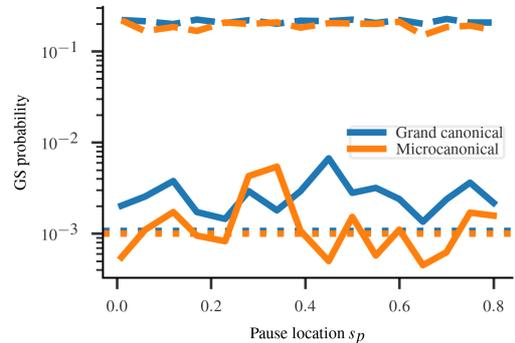
Fig.1 Ground state probability results for the optimization of a Krypton primitive cell using QA (dotted), QA+pausing (solid) and QA+pausing+BFGS (dashed) plotted against the pause location. Grand canonical is with density optimization, microcanonical without.
