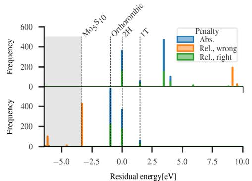
Fig.2 Histogram of obtained configurations using fixed ratio of species (Rel. penalty) or fixed number of atoms (Abs. penalty). The top histogram is SA while the bottom is SA+BFGS. The orange energies have the wrong densities while the green ones the correct density.
