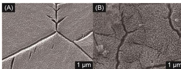
Fig. 2 SEM micrographs of the surfaces of the HAp thin films fabricated via the crystallization under the solution condition (A) I and (B) II.
