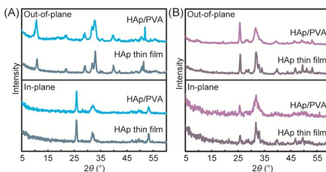
Fig. 1 XRD spectra of the HAp/PVA hybrids and HAp thin films prepared via the crystallization under the solution condition (A) I and (B) II.
