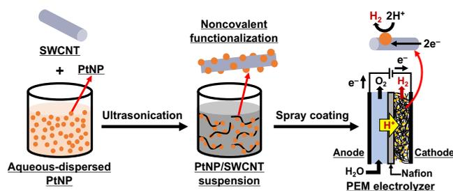
Fig.1 PEM electrolyzer for H<sub>2</sub> production using a PtNP/SWCNT suspension prepared through noncovalent functionalization.
