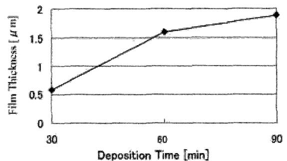
Fig. 5 Dependence of film thickness on deposition time
