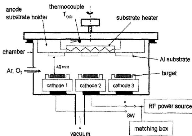
Fig. 3 Magnetron sputtering apparatus
