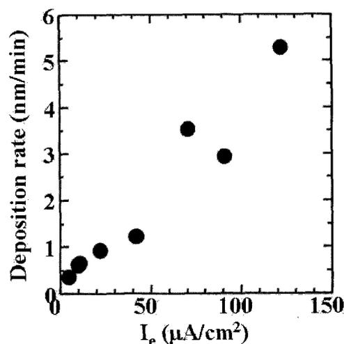
Fig. 2. Dependence of deposition rate on  $I_e$ .
