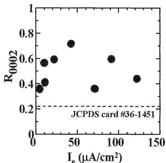
Fig. 4. Electrolytic current density dependence of the preferred orientation tendency parameter.
