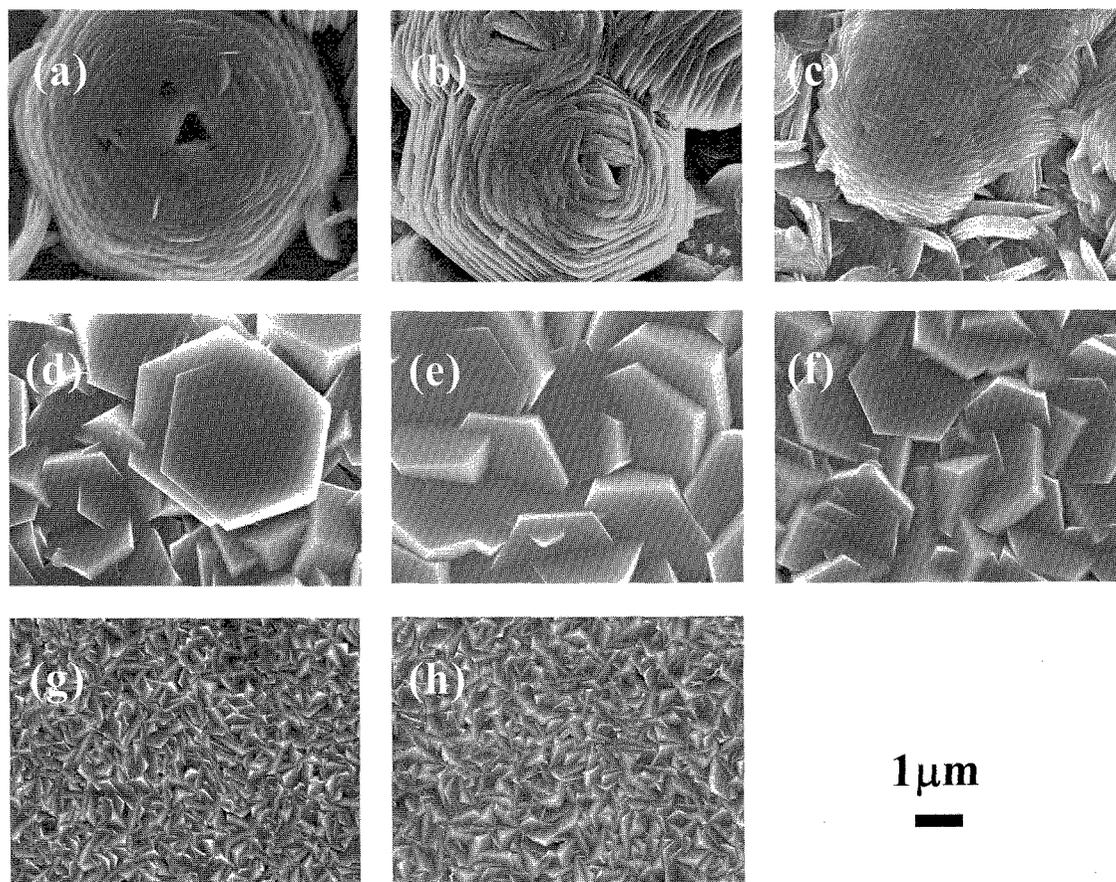
Fig. 5. SEM images of ZnO films prepared with  $I_e$  of (a); 4.5, (b); 9.9, (c); 11, (d); 22, (e); 42, (f); 71, (g); 91 and (h);  $122 \mu\text{A}/\text{cm}^2$ . Magnification ratios of all images are unified.
