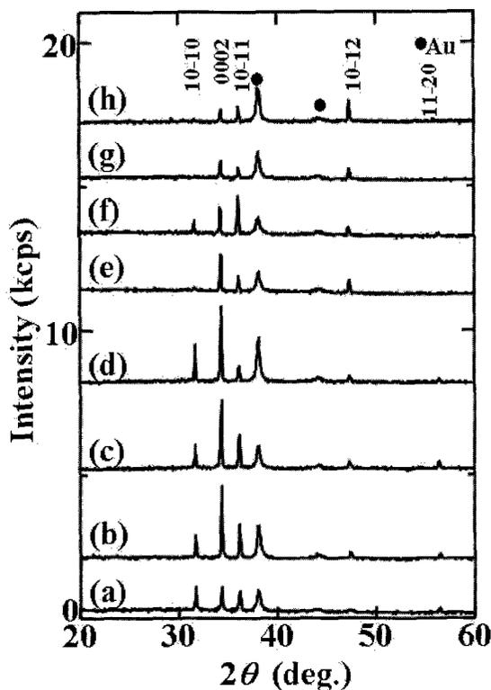
Fig. 3.  $\theta$ - $2\theta$  scan XRD patterns from ZnO films prepared with  $I_e$  of (a); 4.5, (b); 9.9, (c); 11, (d); 22, (e); 42, (f); 71, (g); 91 and (h); 122  $\mu\text{A}/\text{cm}^2$ . The filled circles indicate diffractions from Au as substrate.
