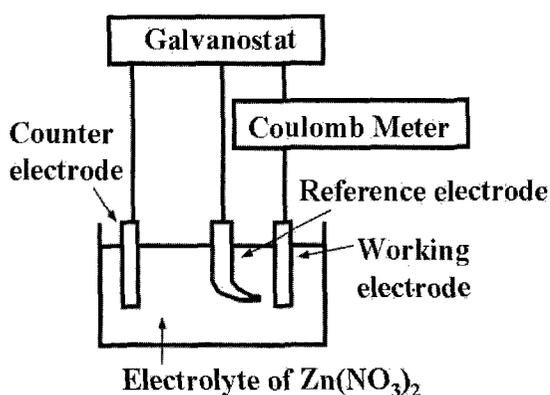
Fig. 1. A schematic view of the equipment for the electrochemical deposition method.
