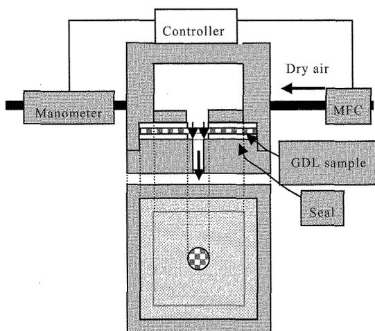
Fig. 3. Schematic diagram of equipment for dehydration pressure test
