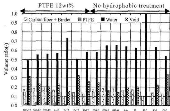
Fig.6. Volume ratio of water impregnated GDLs
