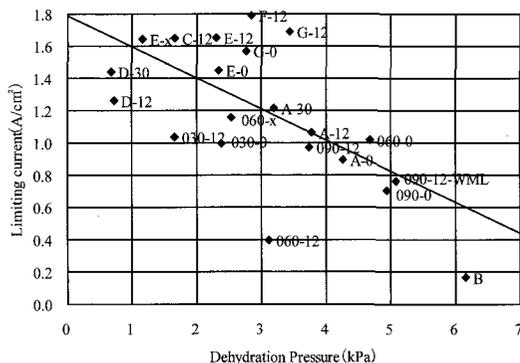
Fig. 7. Limiting current as function of dehydration pressure
