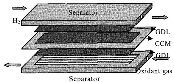
Fig. 1. Cell configuration
