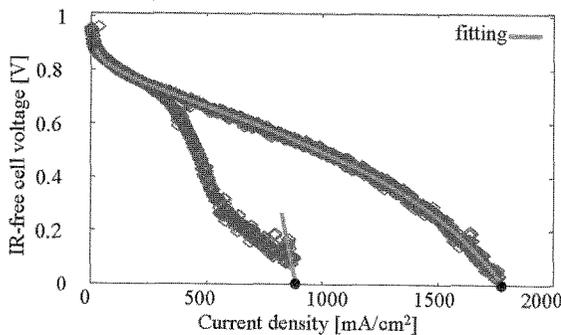
Fig.5. Demonstration of limiting current determination
