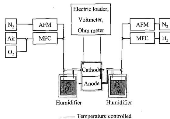
Fig. 2. Schematic diagram of equipment for power generation tests and diagnostic measurements. AFM shows Area flow meter and MFC shows mass flow controller.
