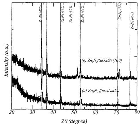
Fig. 3. XRD pattern of  $Zn_3N_2$  on different substrates
