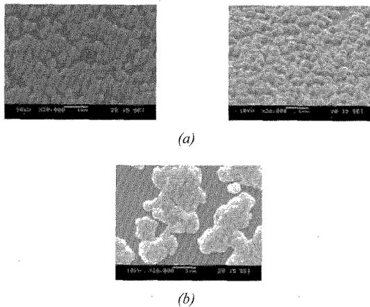
**Fig. 4.** SEM images of  $Zn_3N_2$  on different substrates
