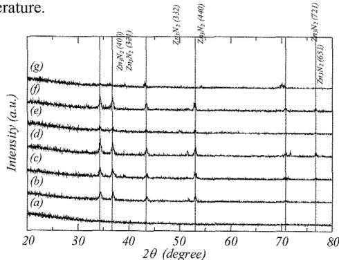
Fig. 1. XRD patterns of  $Zn_3N_2$  / Si (100) obtained at various growth temperatures
