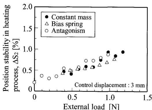
**Fig. 11 Relationship between the positional stability  $\Delta S_2$  and the external load at the control displacement of 3mm.**
