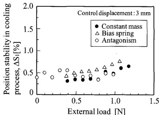
**Fig. 10 Relationship between the positional stability  $\Delta S_1$  and the external load at the control displacement of 3mm.**
