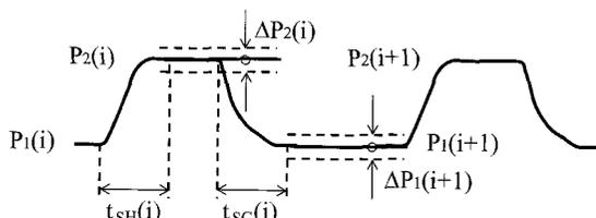
Fig.3 Measurement of settling velocity, position error, and position stability.
