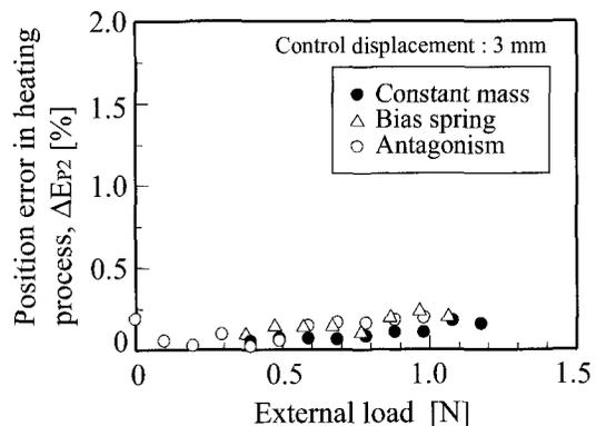
Fig. 9 Relationship between the positional error  $\Delta E_{P2}$  and the external load at the control displacement of 3mm.
