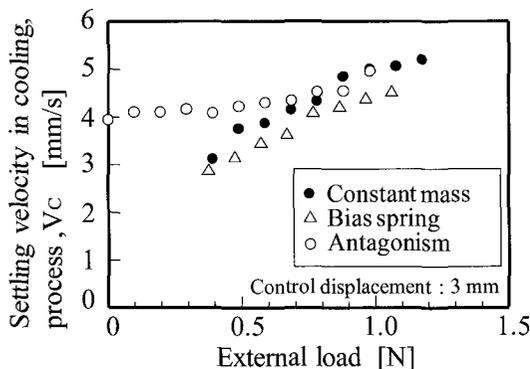
Fig. 7 Variation of the settling velocity  $V_C$  with the external load at the control displacement of 3mm.
