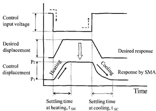
Fig.2 Variation of control displacement with time.
