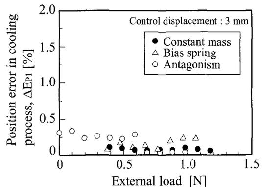
Fig. 8 Relationship between the positional error  $\Delta E_{P1}$  and the external load at the control displacement of 3mm.
