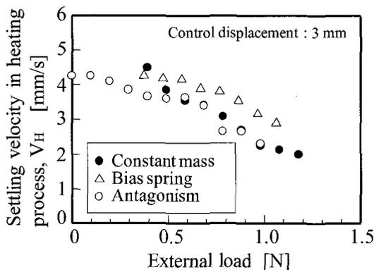
Fig. 6 Variation of the settling velocity  $V_H$  with the external load at the control displacement of 3mm.
