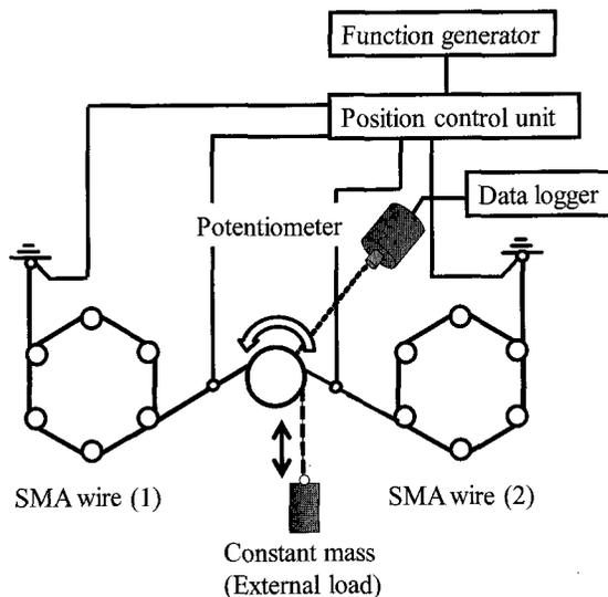
Fig.1 A schematic diagram of antagonism type position control system.
