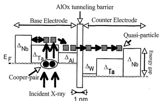
Fig.3 New structure of STJ device to improve the production-collection efficiency of quasi-particles.
