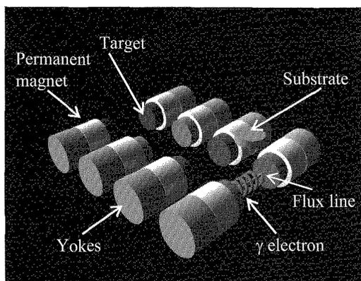
Fig.4 A schematic diagram of total cathode in the case of 4-target sputtering constituted by the conventional FTS system
