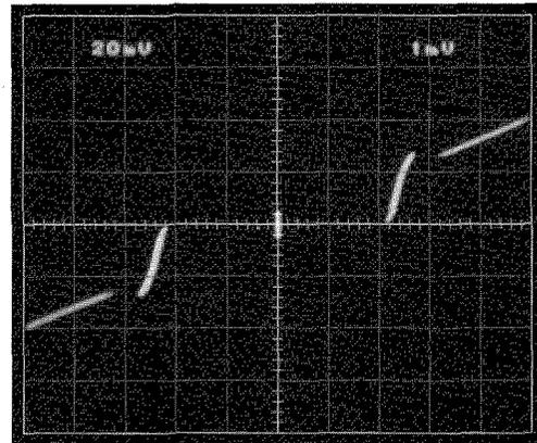
Fig.2 I-V characteristics of STJ device fabricated using the conventional FTS sputtering system, measured at 4.2 K.
