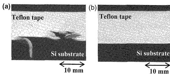
Fig.1 Damage to the Teflon tape placed on the Si substrate during the deposition of the SiO<sub>2</sub> film.
