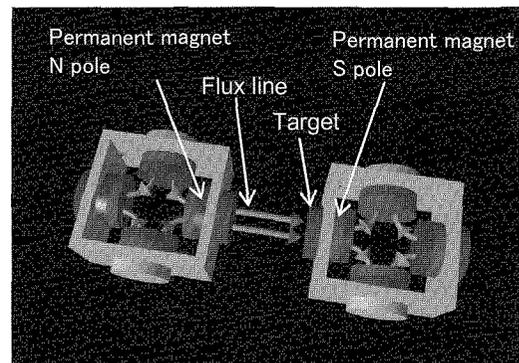
Fig.5 A schematic diagram of a novelty rotating box type multi-facing target sputtering
