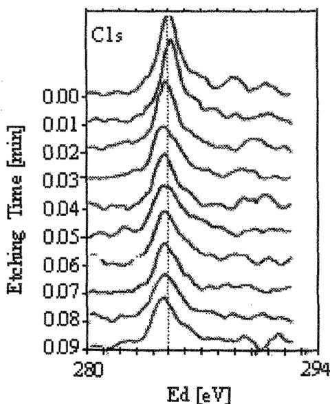
Figure 1 : C1s XPS spectra of C60 thin film
