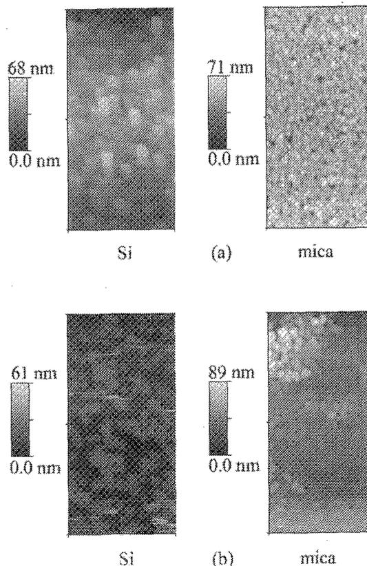
Figure 2 : AFM images on Si and mica substrates grown at (a) 100 °C and (b) 200 °C in  $T_s$ . The size of the photographs is 5  $\times$  2.5  $\mu\text{m}$ . The height gauge is set at the left side of the each photograph.
