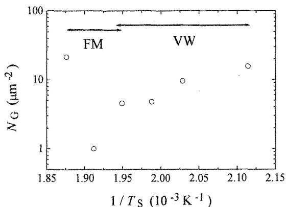
Figure 4 : Arrhenius plot of the number of grains per unit area,  $N_G$ .
