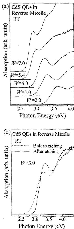
Fig. 5. (a) Absorption spectra for CdS QDs grown in reverse micelles with various values of water contents ( $W=2.0, 3.0, 4.0, 5.4,$  and  $7.0$ ). (b) Absorption spectra for CdS QDs with  $W=3.0$  before (broken line) and after (solid line) the photoetching treatment.
