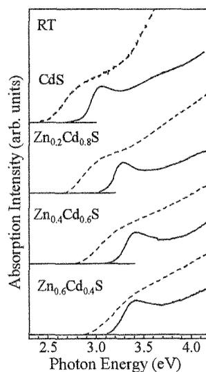
Fig. 4. Absorption spectra for  $Zn_{1-x}Cd_xS$  QDs ( $x=0.4, 0.6, 0.8,$  and 1) in PVP solutions before (broken lines) and after (solid lines) the size-selective photoetching treatment.
