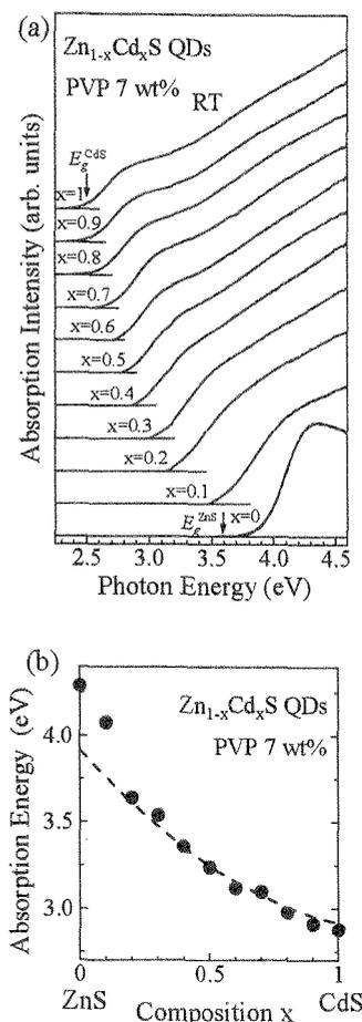
Fig. 3. (a) Absorption spectra for  $Zn_{1-x}Cd_xS$  QDs grown in PVP aqueous solutions. Down arrows indicate band-gap energies  $E_g^{ZnS}$  ( $E_g^{CdS}$ ) in ZnS (CdS) bulk crystals. (b) Alloy-composition dependence of absorption energies ( $\bullet$ ) for  $Zn_{1-x}Cd_xS$  QDs in PVP solutions. Broken line indicates the calculated result for the lowest optical transition energies in  $Zn_{1-x}Cd_xS$  QDs with a radius of 1.9 nm.
