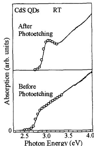
Fig. 2. Absorption spectra for CdS QDs in PVP solutions before and after the size-selective photoetching process. Open circles indicate results of the line-shape analysis.
