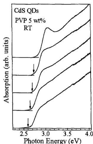
Fig. 1. Absorption spectra for CdS QDs in PVP solutions during a size-selective photoetching process. Down arrows indicate the energy positions of the irradiated monochromatic light.
