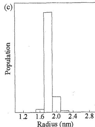
Fig. 6. (a) Absorption spectrum for CdS QDs in the reverse micelle with  $W=5.4$  (b) TEM image of the CdS QD. (c) Size distribution of CdS QDs obtained from TEM images.
