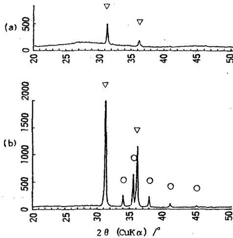
Fig.10. XRD patterns of (a)glass #8 and (b)SiC/glass #8 mixture fired at 800°C for 10min. ○:SiC and ▽:Pb.
