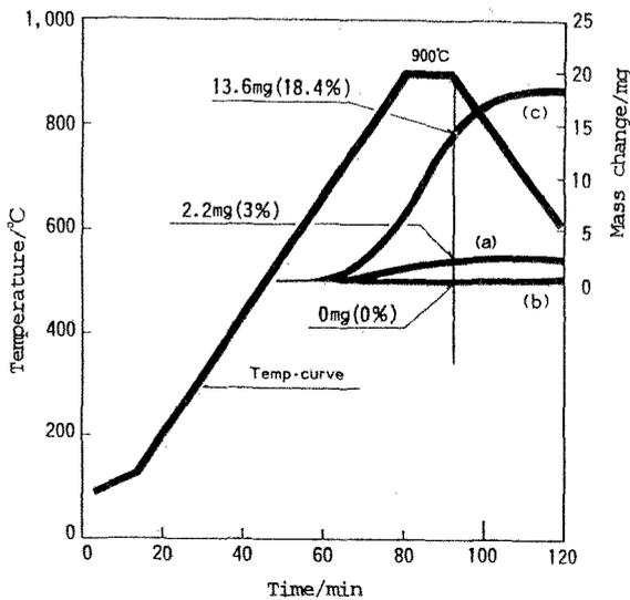
Fig.1. T.G. analysis curves of (a)SiC powder, (b)glass powder, and (c) mixture of SiC(74mg)/Glass (95mg).
