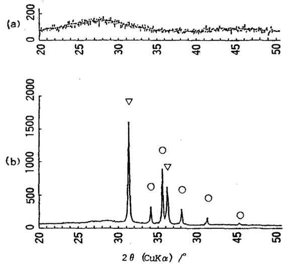
Fig.12. XRD patterns of (a)glass #10 and (b)SiC/glass #10 mixture fired at 800°C for 10min. ○:SiC and ▽:Pb.
