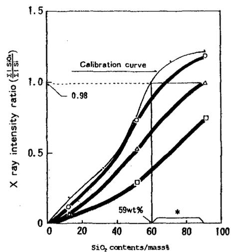
Fig.13. Relationship between SiO<sub>2</sub> content in glass #5 and XRD intensity ratio ( $I_{SiO_2}/I_{Si}$ ) as a function of fusion temperatures. ○:fused at 700°C for 30 min, △:fused at 900°C for 30 min and □:fused at 1100°C.
