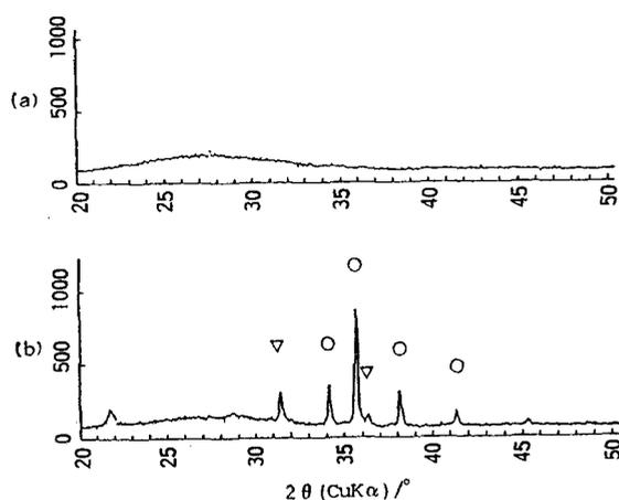
Fig.7. XRD patterns of (a)glass #7 and (b)SiC/glass #7 mixture fired at 900°C for 10min. ○:SiC and ▽:Pb.
