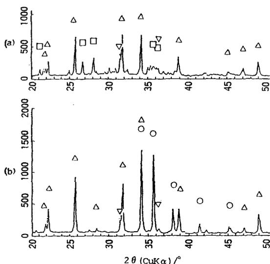
Fig.5. XRD patterns of (a)glass #5 and (b)SiC/glass #5 mixture fired at 900°C for 10min. ○:SiC, △:Zn<sub>2</sub>SiO<sub>4</sub>, □:Zn<sub>3</sub>(BO<sub>3</sub>)<sub>2</sub> and ▽:Pb.
