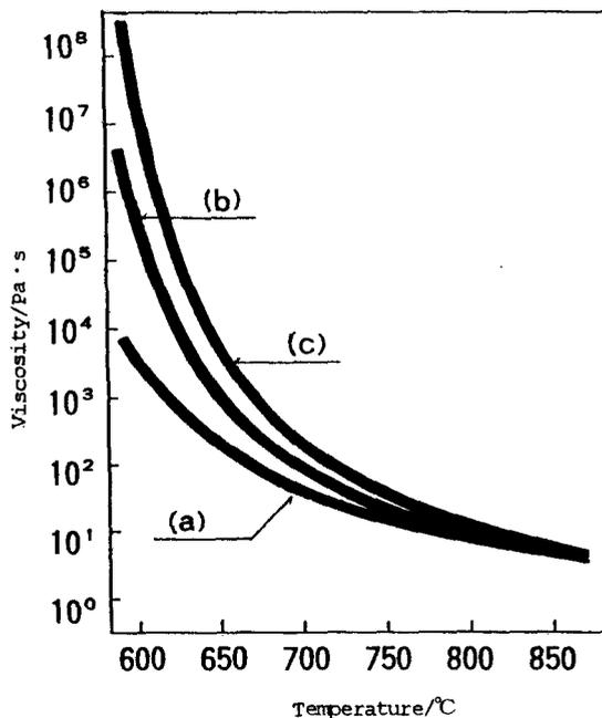
Fig.9. Viscosity of lead boro silicate glasses with various amount of Al<sub>2</sub>O<sub>3</sub> (a)glass #8(Al<sub>2</sub>O<sub>3</sub> free), (b)glass #9(3 mass% Al<sub>2</sub>O<sub>3</sub>) and (c)glass #10(6 mass% Al<sub>2</sub>O<sub>3</sub>) at temperature range from 600°C to 870°C.
