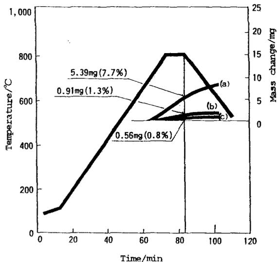
Fig.8. T.G. analysis curves of SiC/glass mixtures composed of lead boro silicate glass with various amount of Al<sub>2</sub>O<sub>3</sub> (a)glass #8(Al<sub>2</sub>O<sub>3</sub> free), (b)glass #9(3 mass% Al<sub>2</sub>O<sub>3</sub>) and (c)glass #10(6 mass% Al<sub>2</sub>O<sub>3</sub>).
