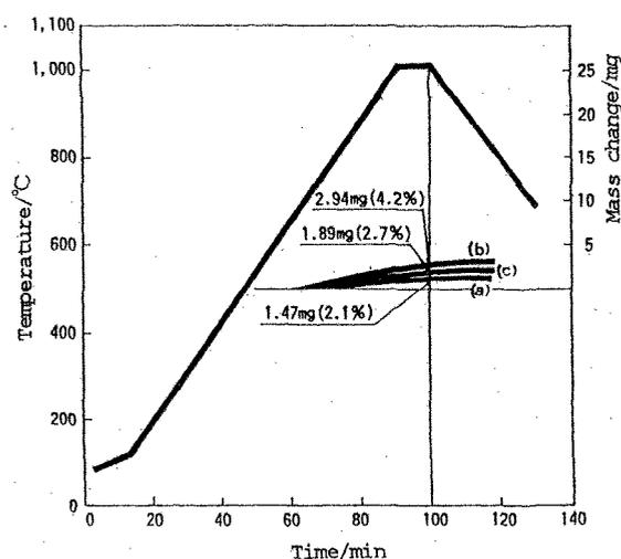
Fig. 15. T.G. analysis curves of SiC/glass mixtures composed of zinc and lead free glass (a)glass #12, (b)glass #13 and (c)glass #14.
