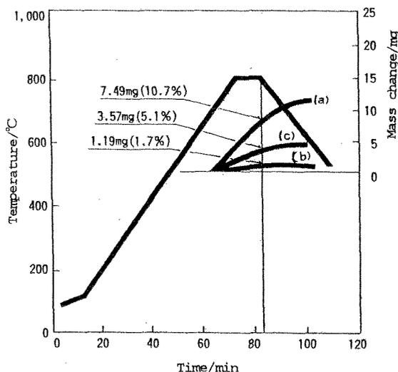
Fig.3. T.G. analysis curves of SiC/glass mixtures composed of three kind of glasses (a)glass #2, (b)glass #3 and (c)glass #4.
