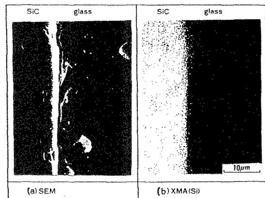
Fig.2. SEM and XMA cross section pictures of glass #1( $\text{SiO}_2$  free glass) film prepared on SiC substrate at 500°C for 10 min.
