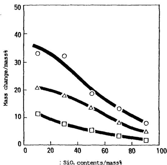
Fig. 14. Percentage mass gain of SiC/glass mixtures composed of various amount of SiO<sub>2</sub> after firing at 900°C for 30min. ○:glass #5, △:glass #6 and □:glass #11.
