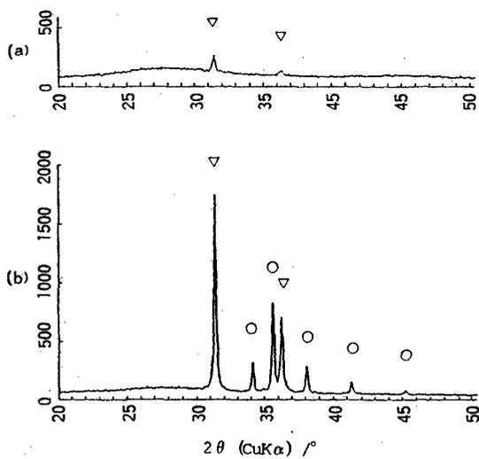
Fig.11. XRD patterns of (a)glass #9 and (b)SiC/glass #9 mixture fired at 800°C for 10min. ○:SiC and ▽:Pb.
