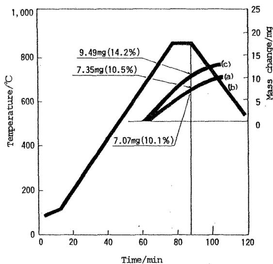
Fig.4. T.G. analysis curves of SiC/glass mixtures composed of three kind of glasses (a)glass #5, (b)glass #6 and (c)glass #7.
