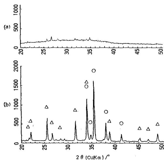
Fig.6. XRD patterns of (a)glass #6 and (b) SiC/glass #6 mixture fired at 900°C for 10min. ○:SiC, △:Zn<sub>2</sub>SiO<sub>4</sub>.
