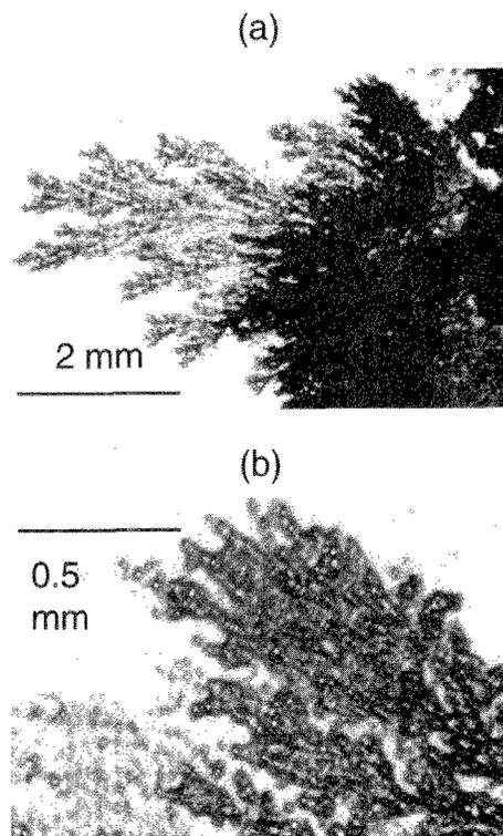
Fig.3 Optical microscope images of the filamentary-breakdown behavior of the MnSb granular film.
