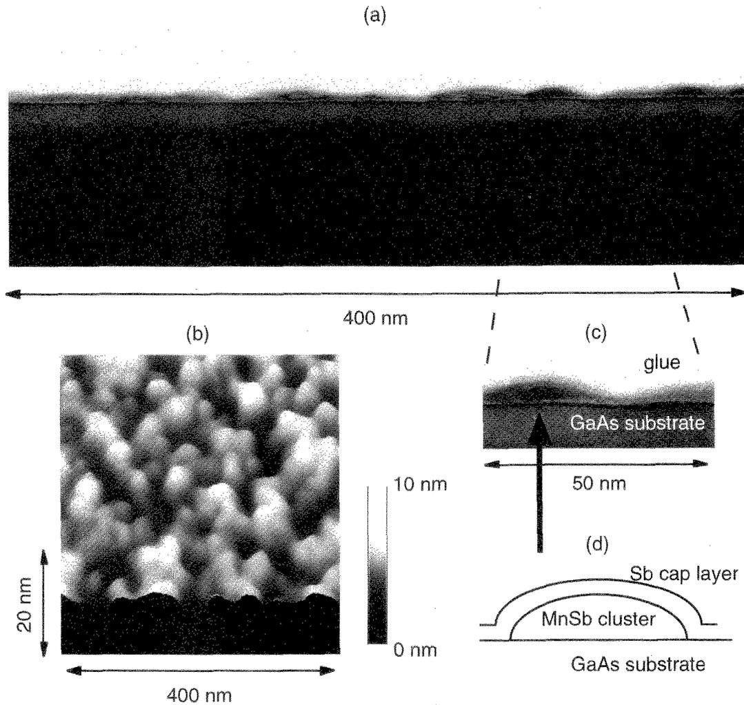
Fig.1 Nanoscale MnSb dots grown on a sulfur passivated GaAs (001) substrate, then covered by a Sb cap layer of 3 nm. (a) Typical cross-sectional transmission electron microscopy (TEM) image of the MnSb granular film. (b) Typical atomic force microscopy image of the MnSb granular film. (c) The magnified cross-sectional TEM image of the MnSb cluster. (d) The schematic drawing of the MnSb cluster grown on the GaAs substrate.
