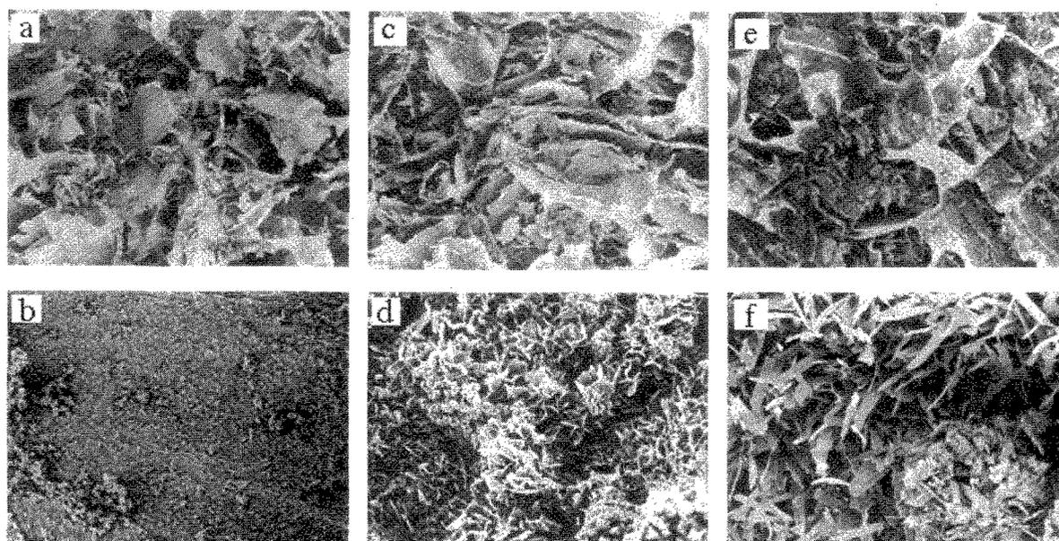
Figure 2. SEM photomicrographs of cross sections of PLGA-collagen-hydroxyapatite composite sponge after 1 cycle of alternate immersion at original magnification  $\times 100$  (a) and  $\times 5000$  (b), 4 cycles at original magnification  $\times 100$  (c) and  $\times 5000$  (d), and 6 cycles at original magnification  $\times 100$  (e) and  $\times 5000$  (f).
