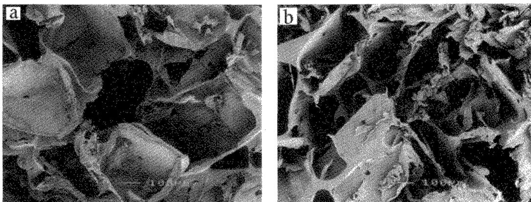
Figure 1. SEM photomicrographs of cross sections of PLGA sponge (a) and PLGA-collagen sponge (b) at original magnification  $\times 100$ .
